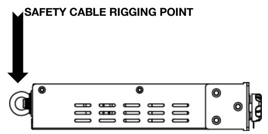
ALWAYS ATTACH A SAFETY CABLE TO THE DEVICE WHENEVER INSTALLING IN A SUSPENDED ENVIRONMENT TO ENSURE THE DEVICE WILL NOT DROP IF CLAMP FAILS.
